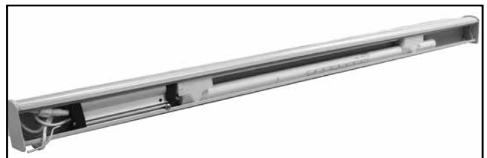
Rechargeable Battery Wand Concealed in Head rail. (Minimum width of 30" required) otherwise battery wand must be mounted externally.
