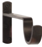
TBKT214-B • 3½"H x ¾"W backplate, 7⅞" front return and 3" back track return* • use to combine 2" or 2¼" full wood pole with single traverse systems • includes traverse ceiling mount bracket attached onto the bottom of the over-bracket
