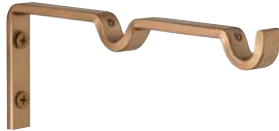
BKT050-2 NEW steel bracket, double 2 1/2" backplate, 6" front return, 3" back return, 1/2"W
